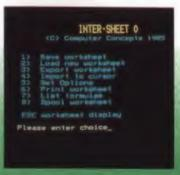
With only one ROM-LINK compatible ROM in the machine then up to 16 sets of data can be held for this ROM. It is a simple matter to switch between sets of data or completely different ROM-LINK programs, and all the data remains in memory intact.
